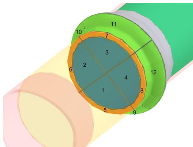
Figure 2 Detailed layout of the membrane at the interface with the concrete
