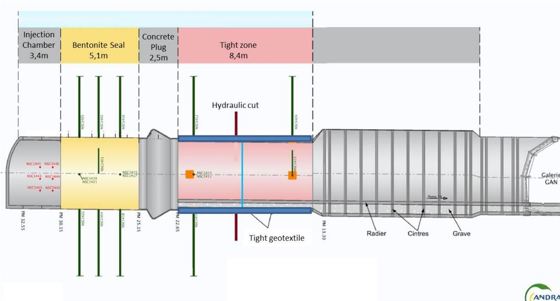
Figure 1 Scheme of NSC experiment
