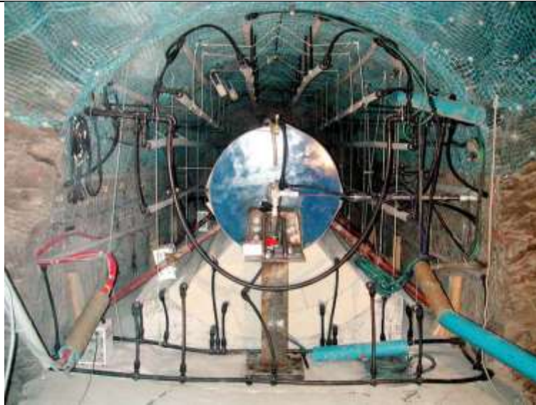
Figure 2: Test elements prior to GBM emplacement and sealing
