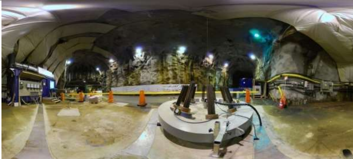
Figure Fel! Ingen text med angivet format i dokumentet. A panoramic view of the Large-scale gas injection test (Lasgit) 420m below ground at the Äspö Hard Rock Laboratory in Sweden.
