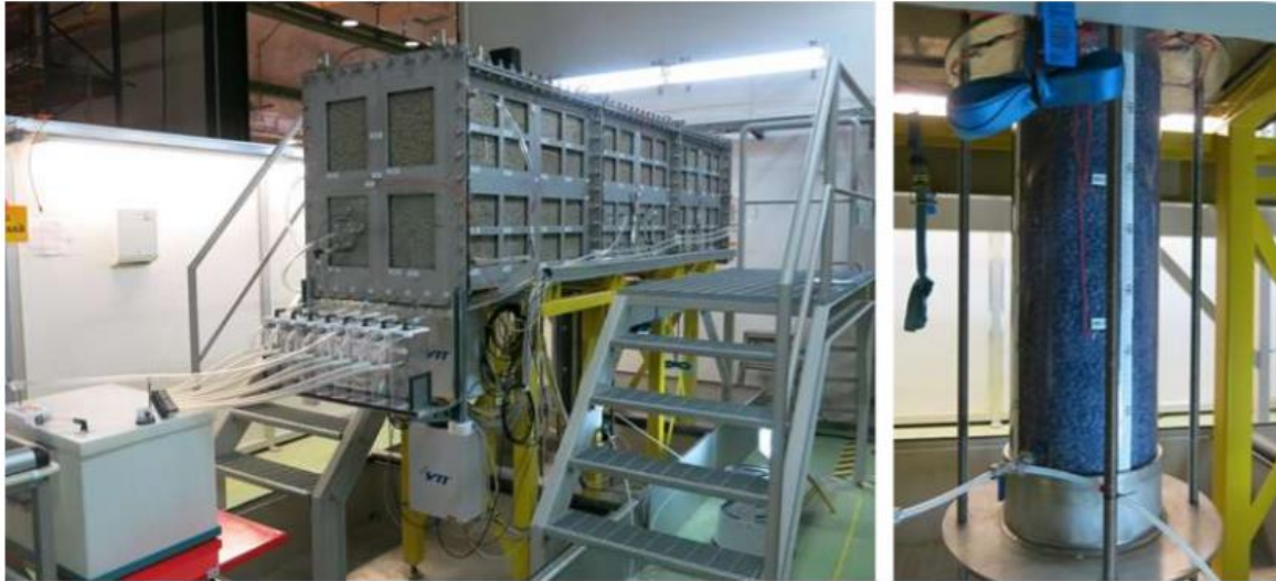
Figure 1. The BBI test equipment simulated the tunnel (left) and the buffer (right) of the KBS-3V concept. The buffer was attached to the bottom of the tunnel.
