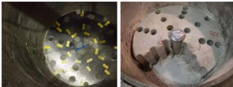
Figure 5. Buffer block 1A during core drilling with a template (left) and block 1J after all samples were taken and first piece of excess bentonite removed showing the dry top face of block 1I (right).
