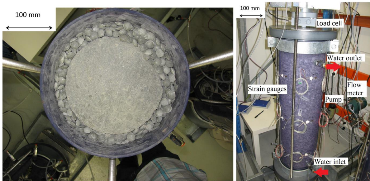
Figure 1. Overhead view of open test assembly showing sample bentonite block and gap filled with bentonite pellets (left). Complete test assembly (right).
