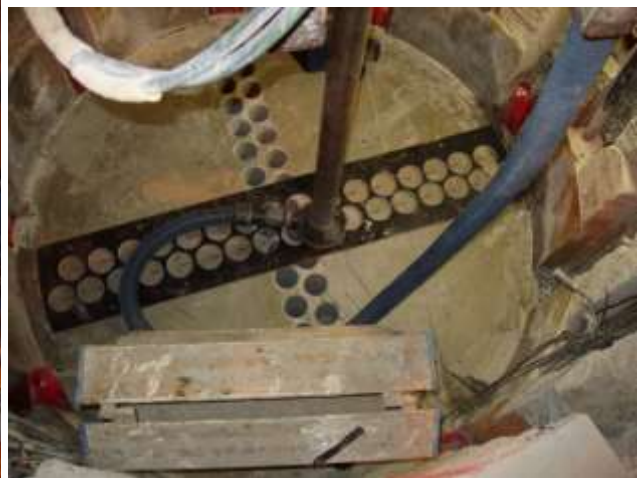
Figure 3. a) The drilling rig placed over the deposition hole. b) Cores taken form the buffer (Johannesson 2007).
